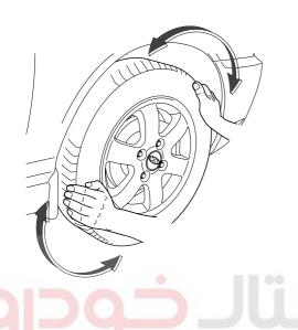
If there is any play, loosen the wheel nuts slightly. Raise the front of the vehicle, and make sure it is securely supported. 3. Remove the front wheel and tire(A) from front hub(B).
