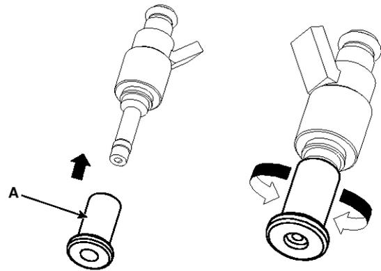
5. Pull the injector out of the sizing tool by turning it in the reverse direction to that used for the press-in process.
