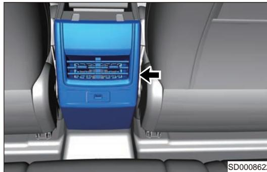
29. Disconnect 1 wire harness connector (arrow) from auxiliary fascia console rear panel assembly, and remove the auxiliary fascia console rear panel assembly.
