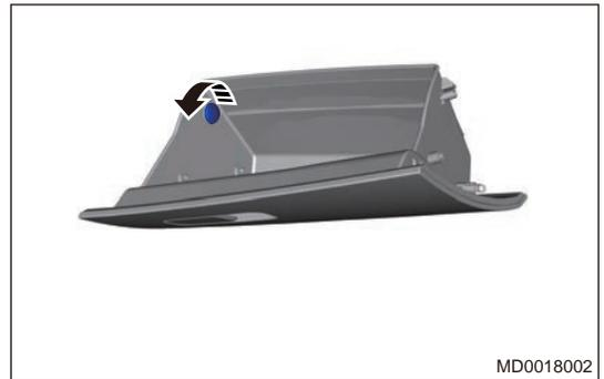
12. Detach the coupling clips between glove box and damper, detach claws from lower side of glove box assembly, and remove glove box assembly (1).
