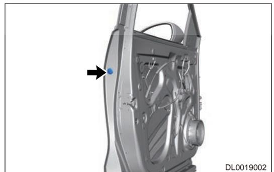
7. Loosen 1 fixing screw (arrow) from front door key cylinder assembly, and remove the front door key cylinder assembly and front door handle protective cover.
