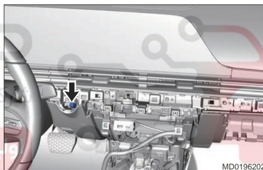
19. Disconnect connector (arrow) from A/C control panel.
