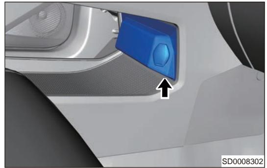
20. Disconnect 3 wire harness connectors (arrow) from storage box block cover.
