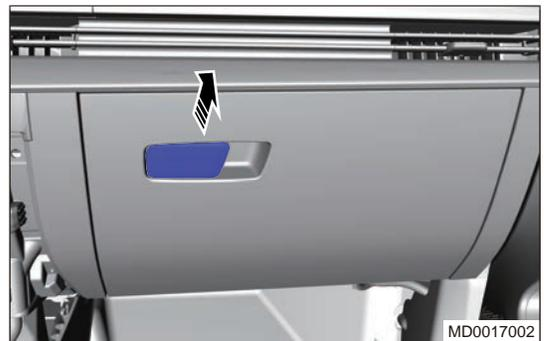
11. Rotate lock knob in direction of arrow as shown in illustration to remove it.
