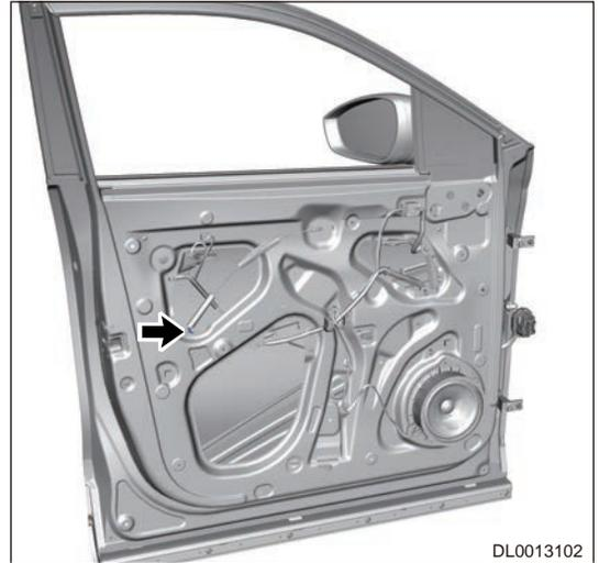
7. Disconnect the connector (arrow) from front left door lock assembly.
