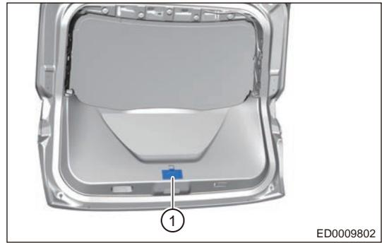
7. Remove the back door lower protector assembly.
