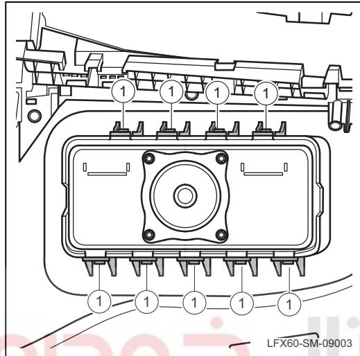
(c). Gently pry the connection tab 1 of occupant airbag and dashboard.
