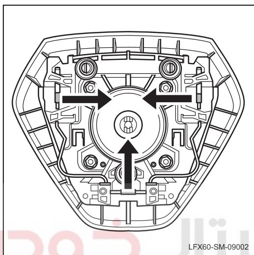
(b). Use the appropriate tool to pry the driver's airbag retainer in the direction of the arrow.
