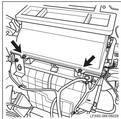
(s). Remove the fixing screws of the upper outlet of HVAC assembly and take it off.
