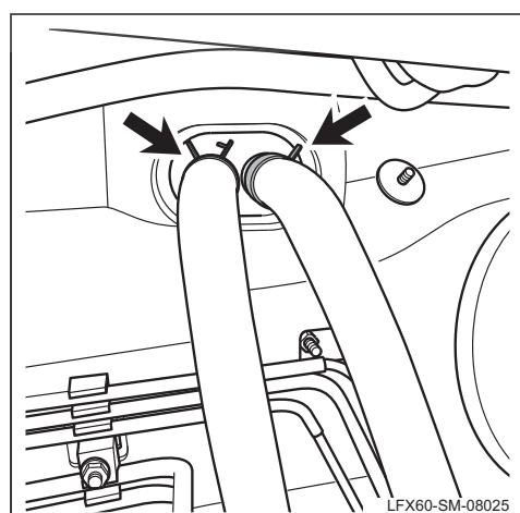
(m). Remove the clamp of heating water pipe.
