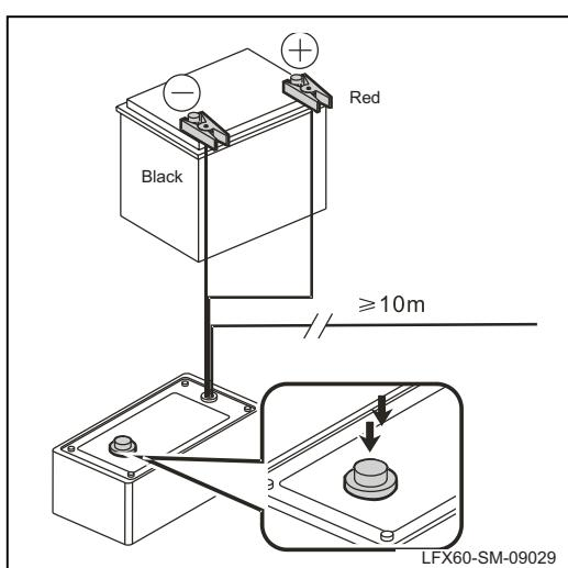
(o). Connect the red and black clamps of the special tools for the airbag detonation to the positive and negative terminals of the backup battery.
