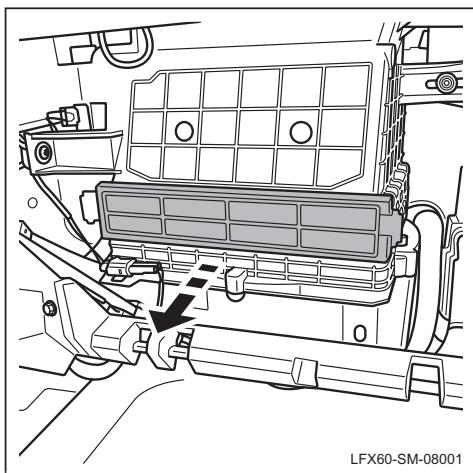
(b) Remove the housing of air conditioning filter and take off the air conditioning filter.
