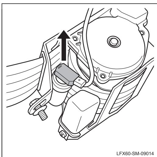
(g). Disconnect the harness plug of seat belt pretensioner.
