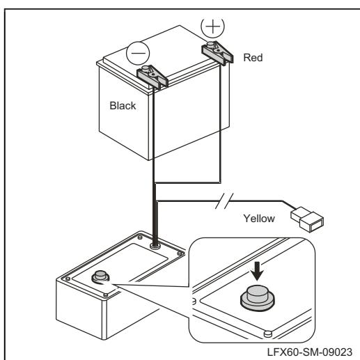
(h). Press down the activation switch of the special tools for airbag detonation to check that if the switch diode lamp is lit.
