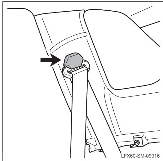
(b). Remove the trim cover of fixing bolts of the seat belt.
