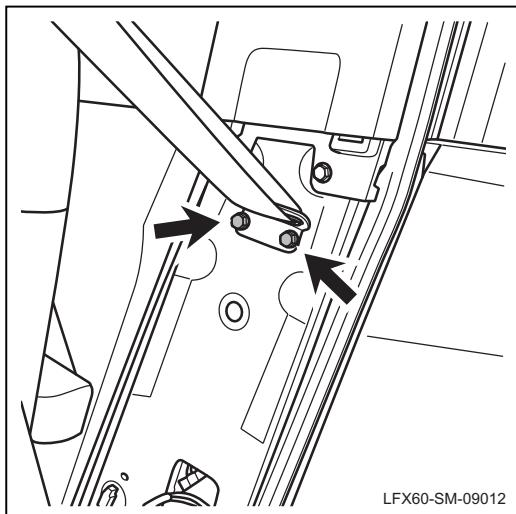
(e). Remove the fixing bolts of stop collar for the front seat belt assembly.
