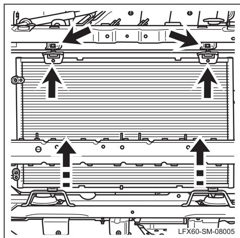
(h). Remove the fixing bolts of the condenser bracket.
