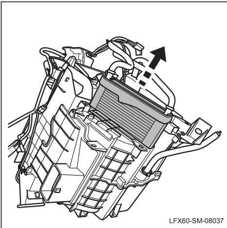
**Installation****1. Install the heating water tank.**
