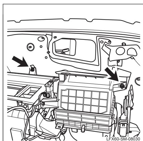
(u). Remove the fixing nut of HVAC assembly.
