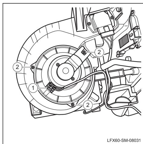
(b). Disconnect the harness connector 1 of blower motor.
