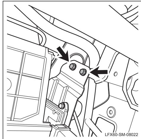
(i). Remove the fixing bolts of the ECU module bracket and the pipe beam.
