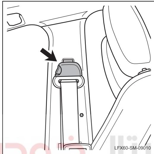
(c). Remove the trim cover of fixing bolts of the front seat belt assembly.
