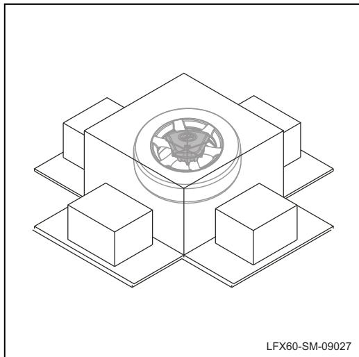
(n). Cover the bundled airbag module with a cardboard box or a used tire.
