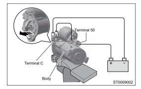
If starter clutch pinion does not move, replace the starter assembly.
