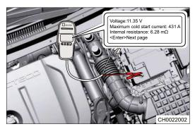
(e) The battery condition is displayed on tester.
