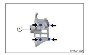
(c) Remove the alternator mounting bracket.
