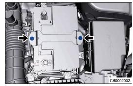
(b) Loosen the locking nuts of positive and negative battery cables, and remove the positive (+) and negative (-) battery cables (1) (2).
