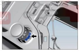
(b) Push fixing clips on both sides of starting switch in direction of arrows and remove starting switch assembly.
