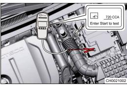
(d) Operate "Left/Right" button on tester to adjust and set the battery capacity (such as 720CCA, this value indicates the battery low temperature starting performance) and click "Enter".
