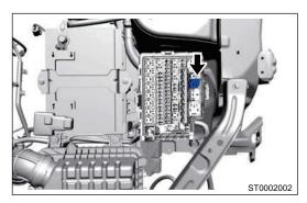
(b) Using a digital multimeter, measure starter relay resistance.
