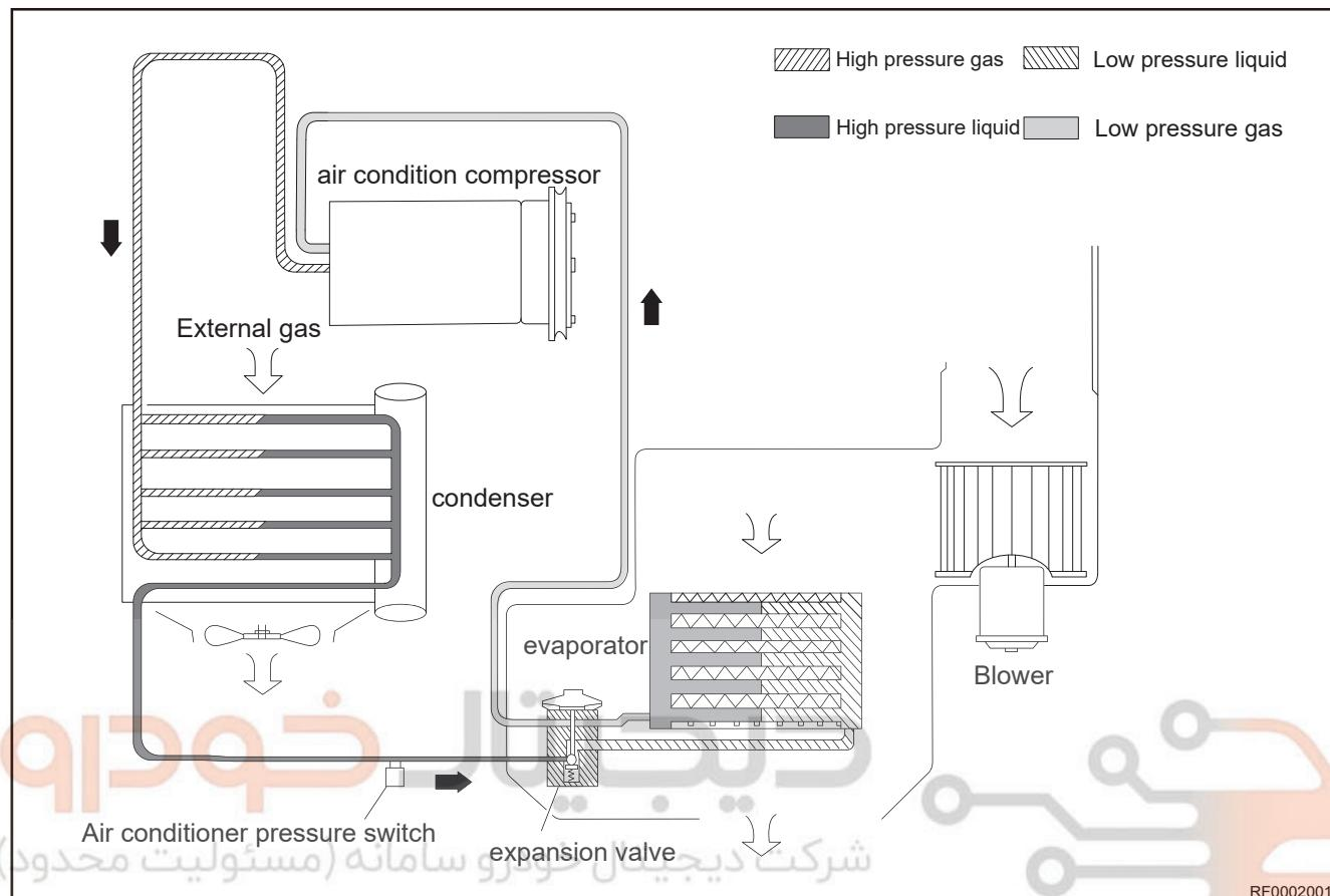
A/C cooling system of vehicle is mainly composed of compressor, expansion valve, condenser, evaporator and blower. The various components are connected by high pressure rubber pipes and steel pipes to form a closed system. When the refrigeration system is operating, the refrigerant circulates in this space in different states. And this cycle is divided into four processes:
