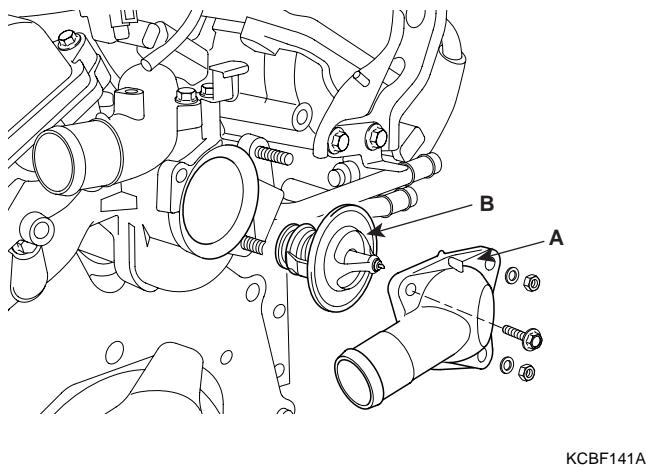
2. Install the coolant inlet pitting(A).
