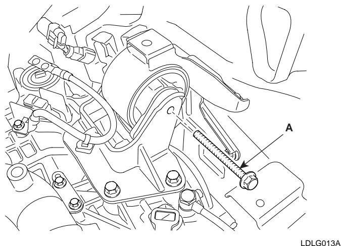
28. Supporting the engine and transaxle assembly with a jack, remove the assembly from the vehicle by loosening the subframe mounting bolts and lifting up the vehicle slowly.
