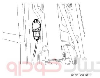
5. Loosen the side impact sensor mounting bolt and remove the side impact sensor.
