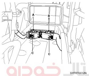
5. Remove the SRSCM mounting nuts from the SRSCM, then remove the SRSCM.
