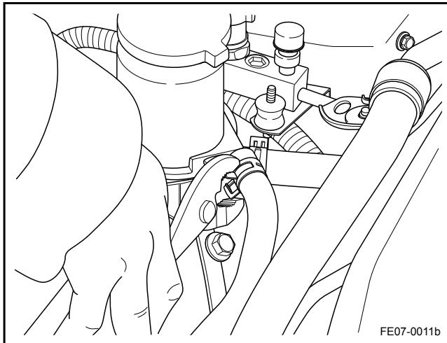
8. Connect the steering system pipe to the fluid reservoir.
