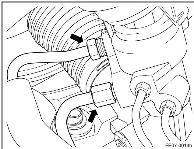
5. Connect the high pressure pipe and the return pipe to the power steering gear and tighten.
