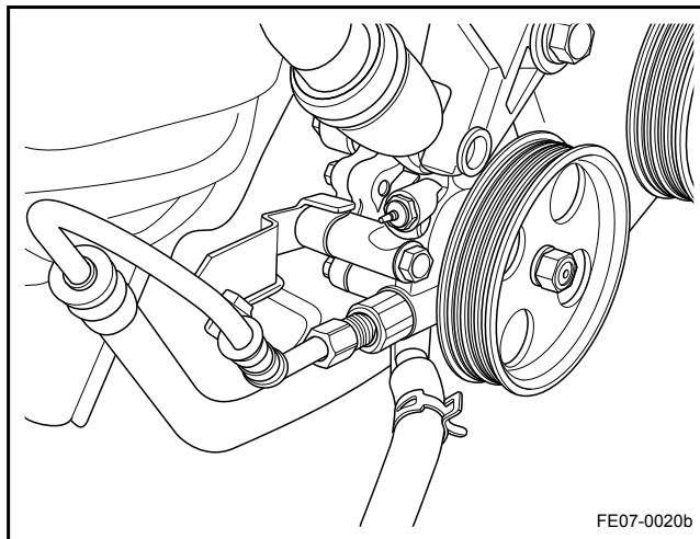
4. Disconnect the high pressure pipe and fluid supply hose from the power steering pump assembly.
