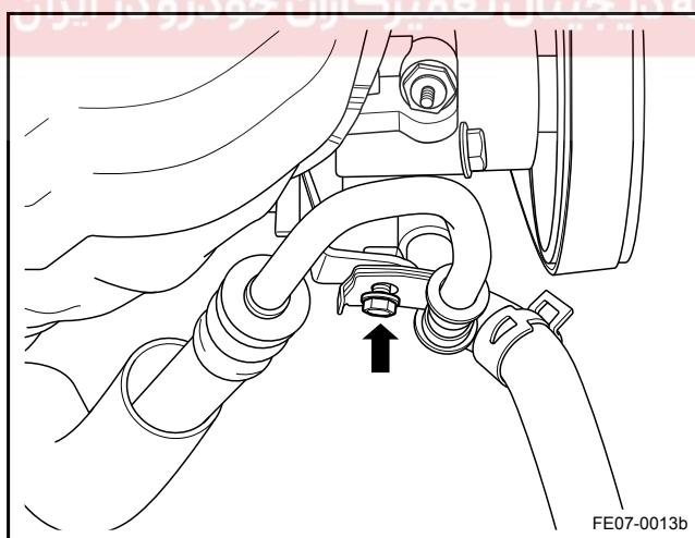
5. Remove the power steering inlet/outlet pipe bracket bolts from the power steering pump assembly.
