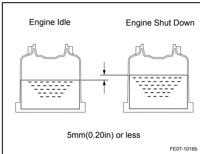
6. With the engine idling, check the fluid level.
