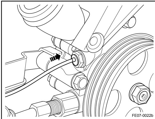
3. Connect the power steering pump pressure switch wiring harness connector.
