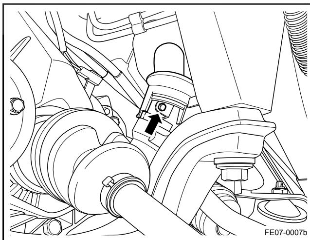
1. Install the mechanical power steering column with the upper and lower steering intermediate shaft assembly to the power steering gear assembly input shaft and tighten the bolts.
