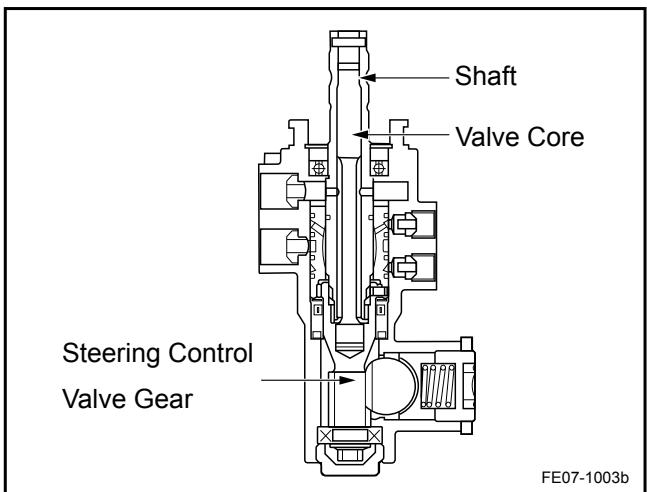
When the steering wheel is not turned, the steering control valve is in the middle position, the master cylinder fluid flows through the steering control valve inlet into the valve cavity. As the steering control valve is in the middle position, so that power cylinder two chamber are connected. The fluid flows from the steering control valve outlet to the fluid reservoir, so the hydraulic power does not work.
