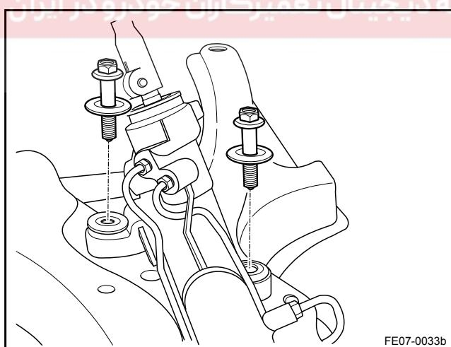
11. Remove the power steering gear to the subframe retaining bolts.
