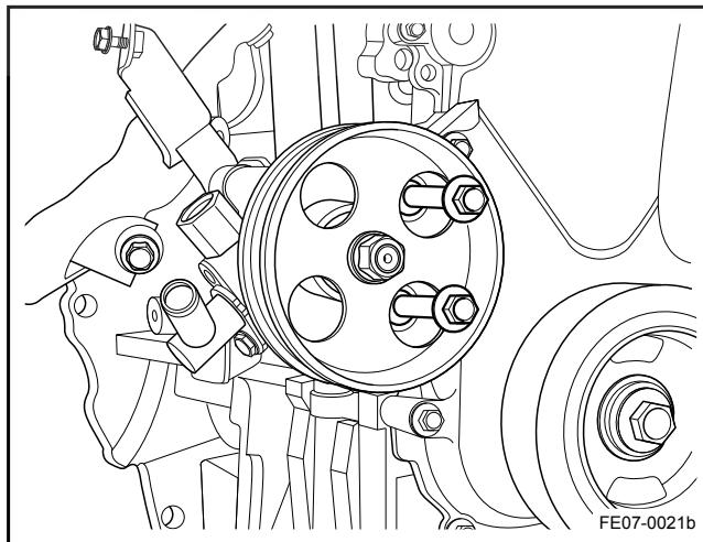
1. Install the power steering pump assembly to the vehicle and tighten the retaining bolts.
