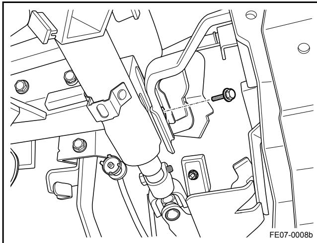
2. Install the mechanical steering column assembly bracket and carrier connecting bolts and tighten.
