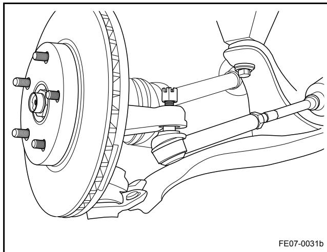
8. Remove the tie rod and the ball joint retaining nut.
