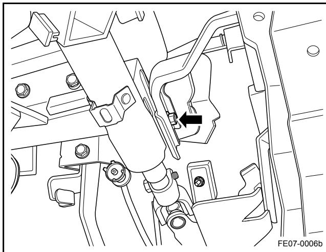
11. Remove the mechanical steering column assembly bracket to carrier connecting bolt.
