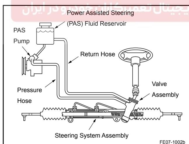
Rack and pinion with hydraulic pressure assistance steering system is as shown in the graphic. The mechanical rack and pinion steering, steering cylinder and steering control valve are designed to be integrated to form the integral power steering system. Power cylinder piston and the rack is made as a whole, the power cylinder is divided into about two chambers.
