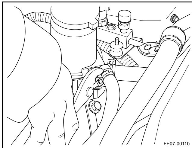
3. Disconnect the power steering outlet pipe from the fluid reservoir.
