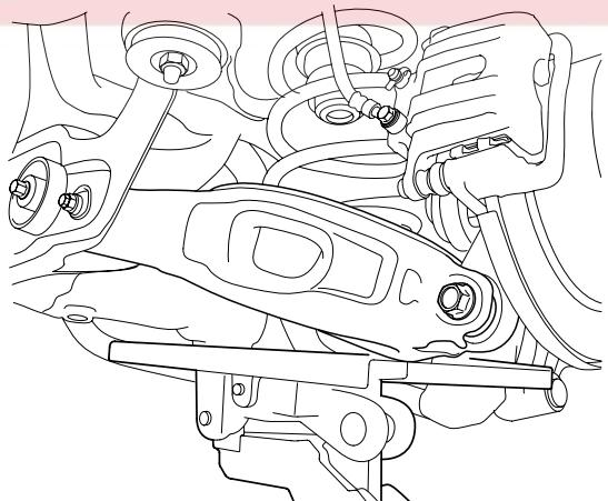
4. Remove the rear shock absorber (A).
