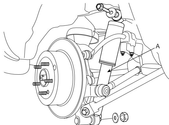
5. Remove the brake caliper mounting bolts (A), and then place the brake caliper assembly (B) with wire as shown in the illustration.
