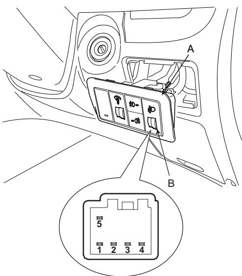
3. Remove the head lamp leveling switch (B) from the lower crash pad switch.
