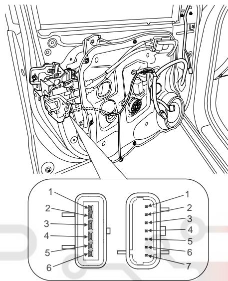
3. Check actuator operation by connecting power and ground according to the table. To prevent damage to the actuator, apply battery voltage only momentarily.
