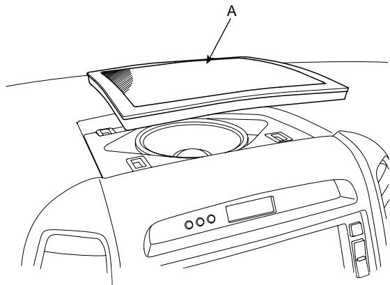
4. Remove the center facia panel(A) after loosening 2 screws. Take care not to damage fixing clips. (Refer to the Body group - Crash pad)
