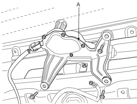
2. Remove the rear wiper cap & pad (B) after removing a nut (A).
