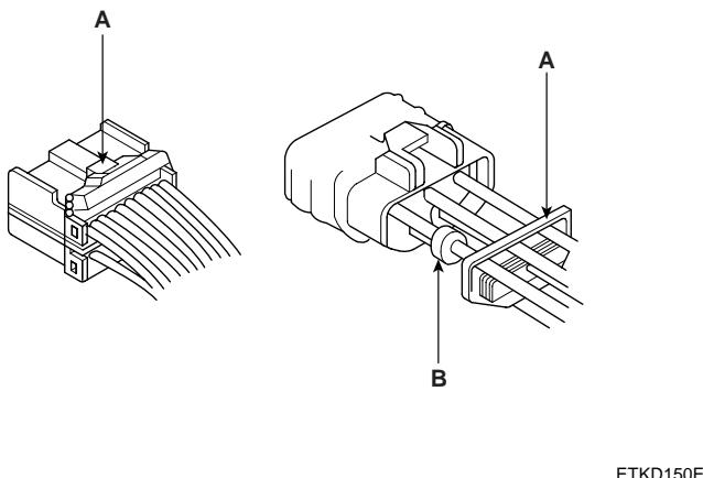
10. The backs of some connectors are packed with grease. Add grease if necessary. If the grease (A) is contaminated, replace it.
