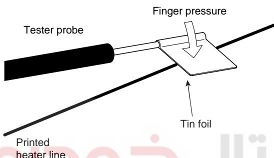
1. Turn on the defogger switch and use a voltmeter to measure the voltage of each heater line at the glass center point. If a voltage of approximately 6V is indicated by the voltmeter, the heater line of the rear window is considered satisfactory.
