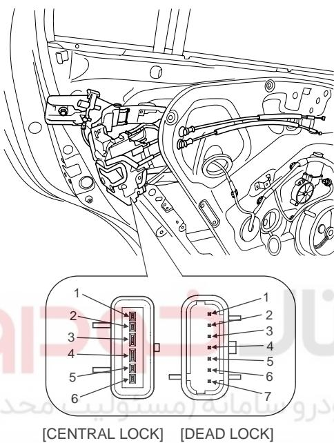
4. Check actuator operation by connecting power and ground according to the table. To prevent damage to the actuator, apply battery voltage only momentarily.
