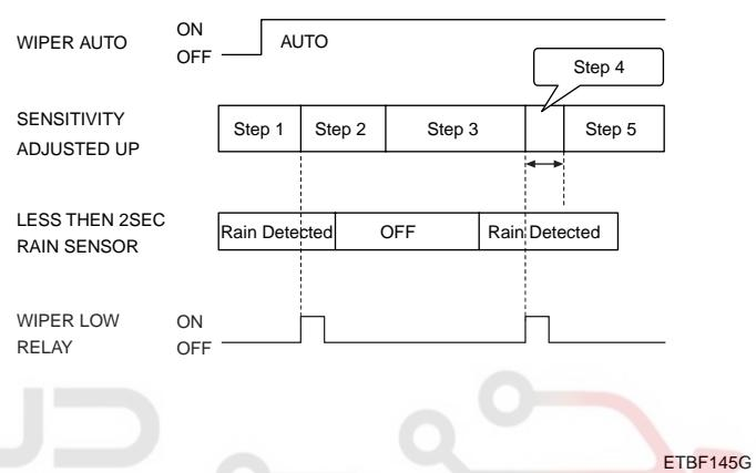
3. A single wipe will be performed whenever rain has been detected (Rain Detected signal from Rain sensor) and the wiper switch is moved to the AUTO position. But a single wipe will not be performed when the wiper switch is moved to the AUTO position and OFF signal is being received from Rain sensor. But if the wiper switch is moved to AUTO position for the first time since vehicle ignition switch is turned on then a single wipe will be performed regardless of Rain Detected or OFF signal.
