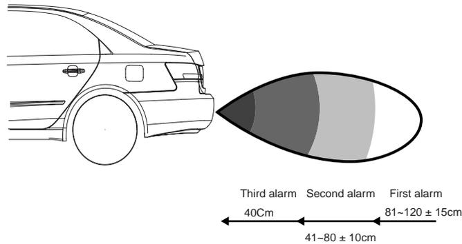
1. Distance tolerance(Messured at the front of sensor)
