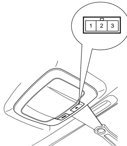
3. Remove the room lamp assembly after removing 2 screws and disconnecting the 3P connector (Standard type). Remove the room lamp assembly by using the scraper and then disconnect the 3P connector (Sun-roof type).
