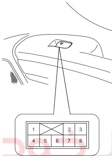
4. Check for continuity between the terminals in each switch position according to the table. If the continuity condition is not normal, replace the switch.
