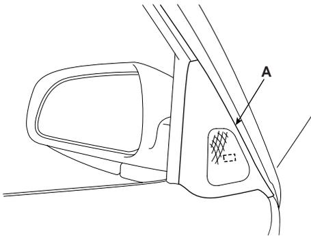
2. Disconnect the power door mirror connector from the harness.
