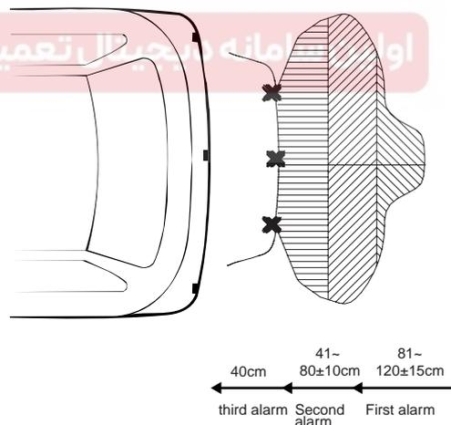
1. Distance tolerance(Messured at the front of sensor)
