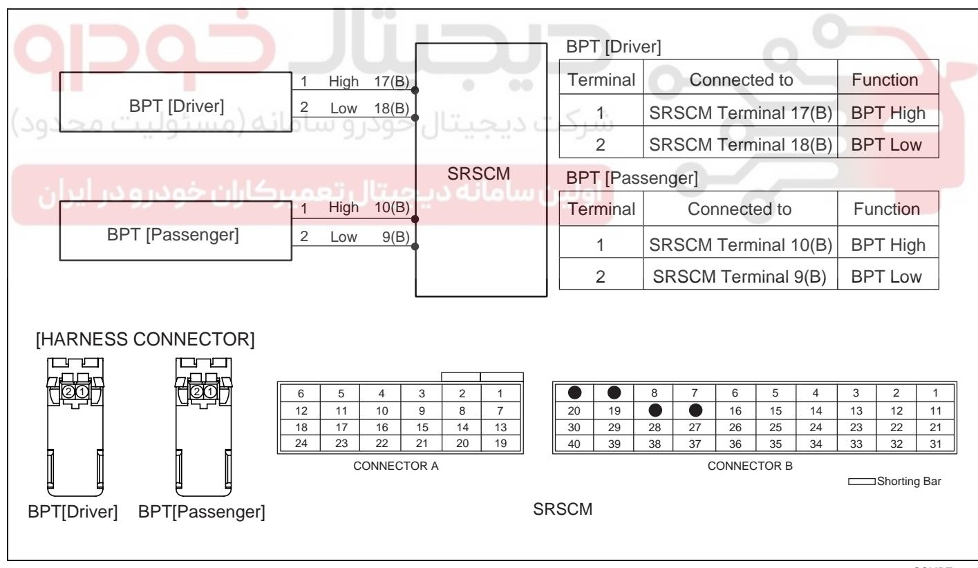
**TERMINAL & CONNECTOR INSPECTION** E61C7A42
